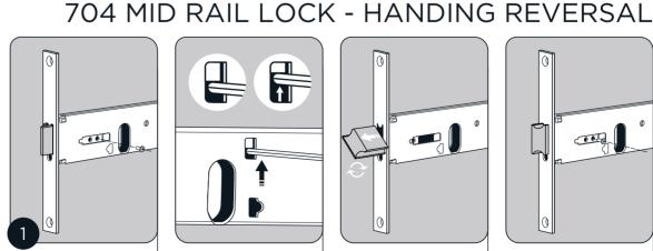
**REMOVE SCREW** Remove the captive screw from the side of the main unit.
