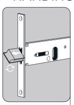
**REPOSITION LATCH** With the latch retainer in the up position, pull the latch out and rotate 180 degrees to reverse the handing, push back into the body and release the latch retainer.
