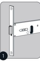
**CHECK HANDING** Determine if handing direction is correct for the door Installation If reversal is needed follow these steps to reverse handing direction.
