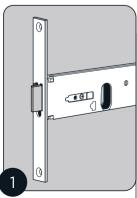
**CHECK HANDING** Determine if handing direction is correct for the door Installation If reversal is needed follow these steps to reverse handing direction.
