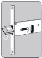
**REPOSITION LATCH** With the latch retainer in the up position, pull the latch out and rotate 180 degrees to reverse the handing, push back into the body and release the latch retainer.
