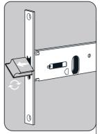
**REPOSITION LATCH** With the latch retainer in the up position, pull the latch out and rotate 180 degrees to reverse the handing, push back into the body and release the latch retainer.
