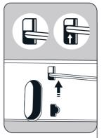
LATCH RETAINER Rotate the assembley and using a thin screwdriver or allen key, raise the latch retainer up as far as it will go.
