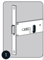
**CHECK HANDING** Determine if handing direction is correct for the door Installation If reversal is needed follow these steps to reverse handing direction.
