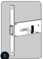
**REMOVE SCREW** Remove the captive screw from the side of the main unit.
