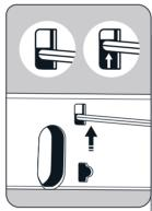
LATCH RETAINER Rotate the assembley and using a thin screwdriver or allen key, raise the latch retainer up as far as it will go.
