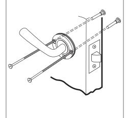
6 Fit cover plates over handles, ensure notch is at the bottom
