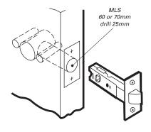
3 Fit spindle through latch
