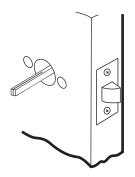
Drill and fit 1x wood screw for alignment only
