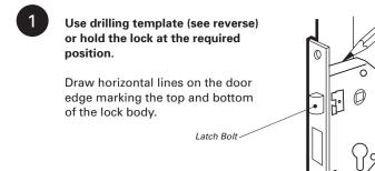
Mark a vertical line at the centre of the door edge between the two horizontal lines.
