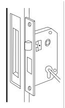
On the door frame, mark the top of the latchbolt and the bottom of the deadbolt.
