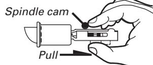
Pull spindle cam all the way to right edge of adjusting hole.
