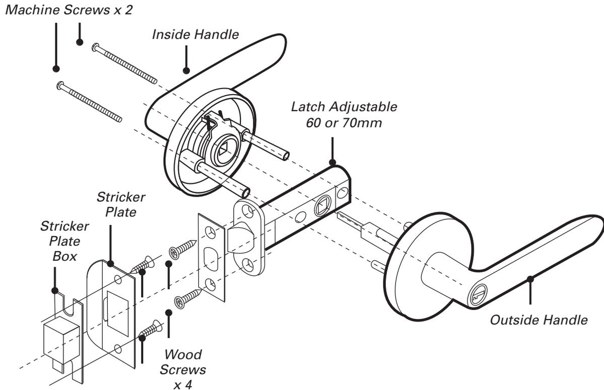
Applicable door thickness ranges from 30mm to 45mm
