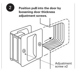
Fit sliding pull handle by tightening adjustment screws ensuring pull is central in the door. Fit the larger style wood screws as shown.
