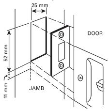
Drill two 15 mm (9/16") diameter holes, 12 mm deep at 20 mm from top of plate to centre of hole and also 35 mm from the top of the plate to the centre of the hole. Chisel out holes to form a rectangular hole for clearance of locking arm.
