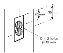
6 Fix striker plate into jamb with the two smaller wood screws provided.
